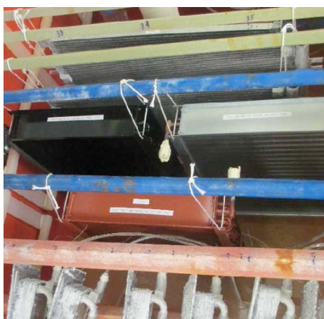
Three test condensers in SWAAT cabinet. Upper left cathodic epoxy coated condenser, upper right bare, un-coated condenser and bottom center immersed/sprayed modified-phenolic coated condenser.
