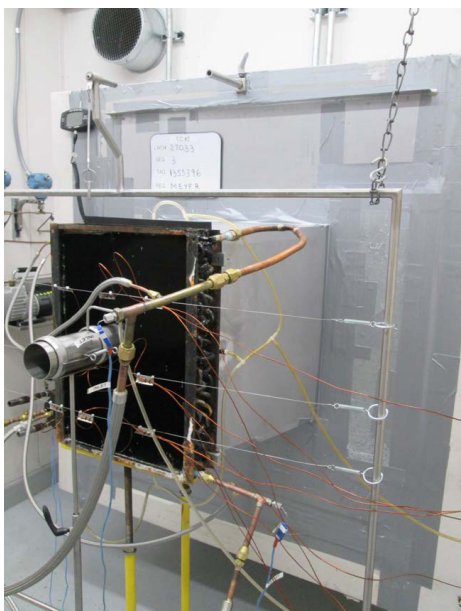
Cathodic epoxy coated condenser shown.
