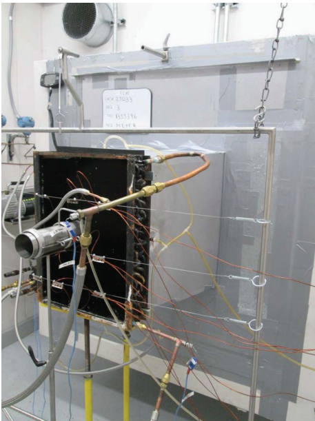
Cathodic epoxy coated condenser shown.
