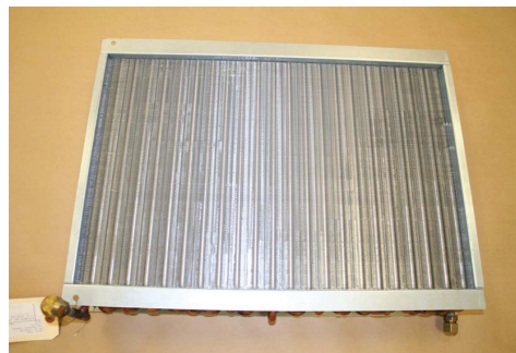
Modine condenser used in coating tests.
